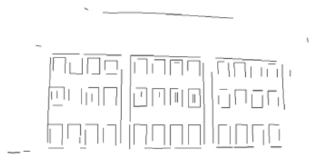
Figure 9: Edge-corner generation process using Indirect Corner Extraction algorithm (ICE)
