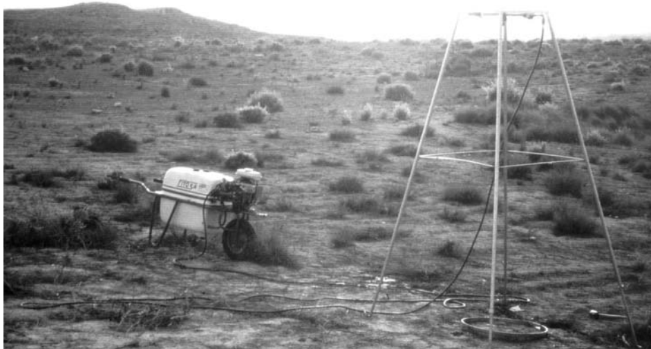
Figure 4. Small mobile rainfall simulator
