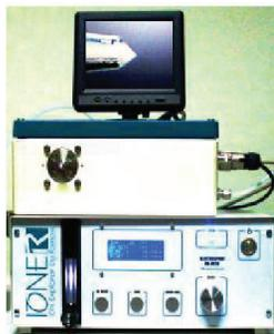
Fluid-electrodynamic device that generates an electrically charged nanoaerosol from a liquid phase sample.
