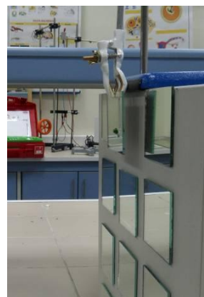
FIGURE 12. One of the 12 pieces of mirror brought forward about 5cm toward the doll, parallel to the other pieces.
