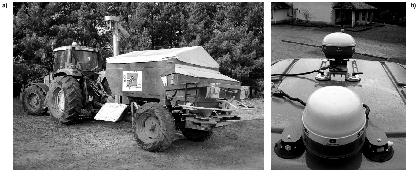
Figure 1. Tractor and trailed twin-disc fertilizer spreader used in trials (a) and location of GPS antennas at the top of the cab (b).
