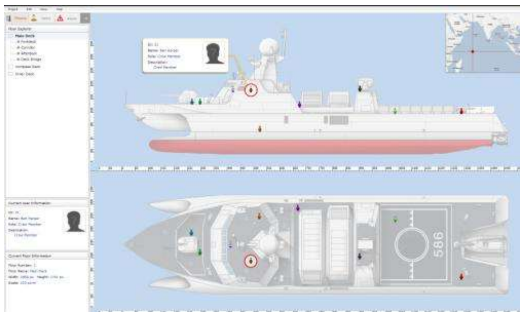
Fig. 3. Web client Graphical user Interface (GUI) of the of the n-Core Polaris RTLS for a maritime scenario.
