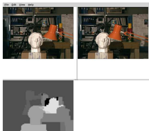
Fig. 5: Interface of the software when placing the image and obtaining the depth information.
