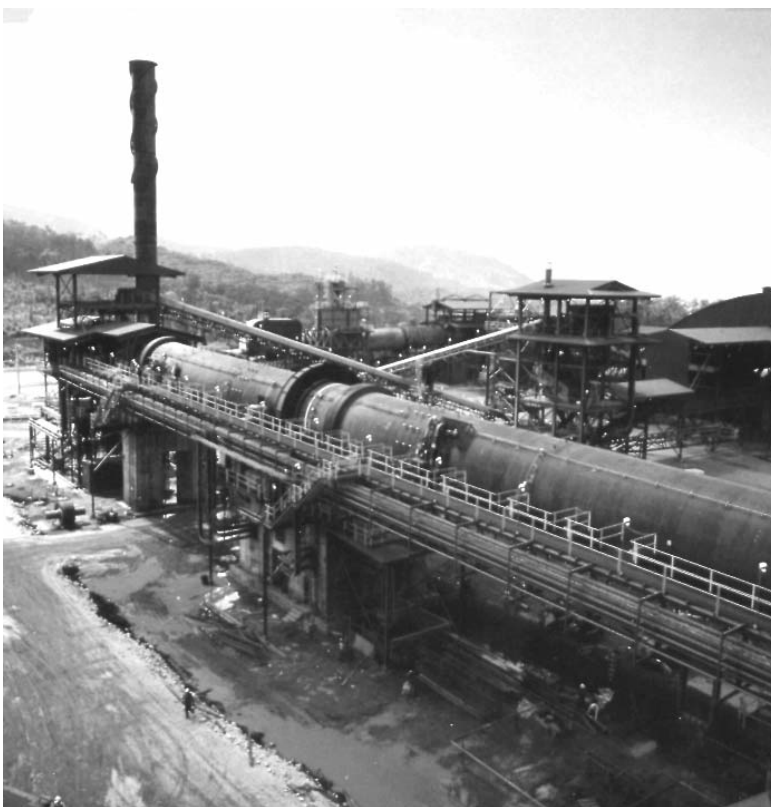
Figure 9. A rotary kiln in a nickel laterite plant.
