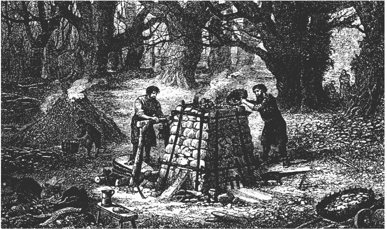
Figure 3. Iron production in Roman times. Note the foot-operated bellows and the charcoal kiln at the left.
