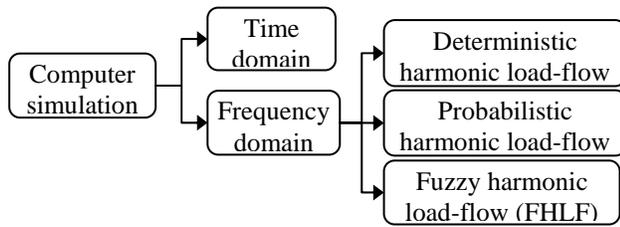
Fig. 1. Different methodologies for harmonic power systems analysis
