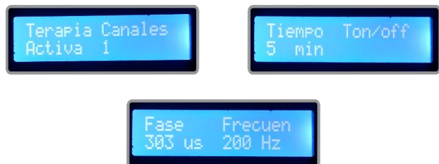
Figure 13. StimFace LCD screen information for active therapy
