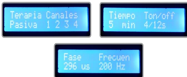
Figure 11. StimFace LCD screen information for passive therapy
