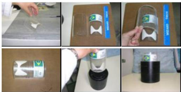
Figure 1. Sequence of preparation for the neck phantom, constructed by the IRD under the ARCAL LXXVII project.
