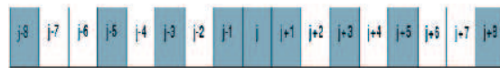
Figure 2. Configuration of the input feature set. Shaded regions indicate the frames in which the log-energy and 12th order PLP features are calculated
