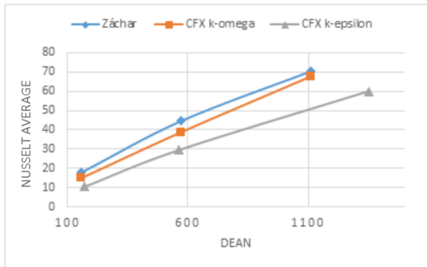
Figure 6 Nu vs. Re, second project, curved corrugated tube, comparison of physical models
