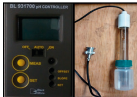
Fig 5. Installed pH. indicator controller. Source: Authors
