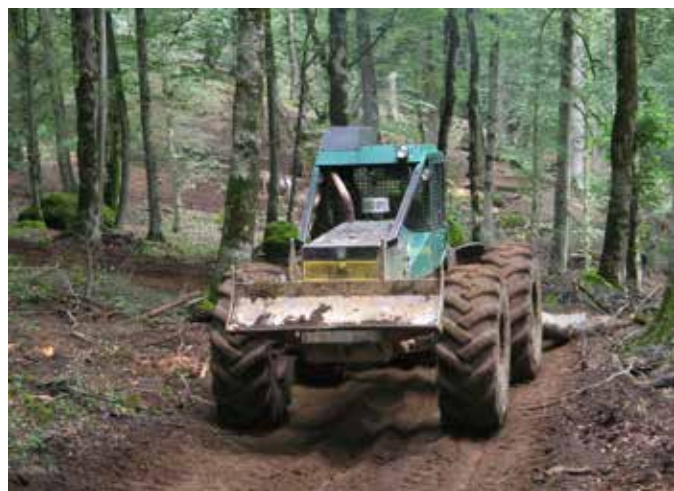
FIGURE 1. Rubber-tired skidder (Timberjack 450C) used in logging operations in a mountain forest of Iran.
