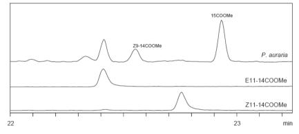
**Figure 4.** Mass chromatogram (m/z 55, base peak of  $\Delta$ 1-14:COOMe) of a derivatized (BF<sub>3</sub>-MeOH) chloroform extract of the pheromone gland of *P. auraria*.
