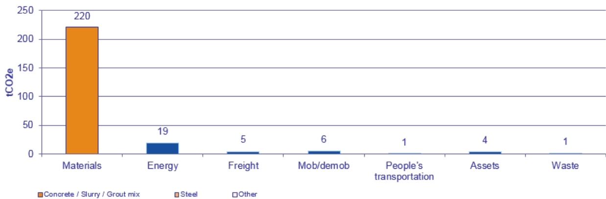
Figure 1- Total carbon footprint divided by the different emission sources evaluated by the carbon calculator (CEM I case)
