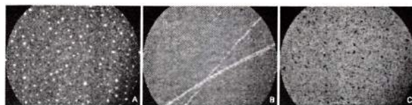
Figure 16. Polystyrene particles on Silicon Wafer, (optical microscope, 50x, dark field). A: 10 °C. B: 15 °C .C: 20 °C
