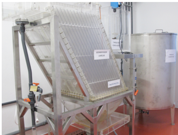
Figure 1. LNECs lamellar sedimentation prototype which will be adapted for pilot trials in two WWTPs (LIFE Impetus).
