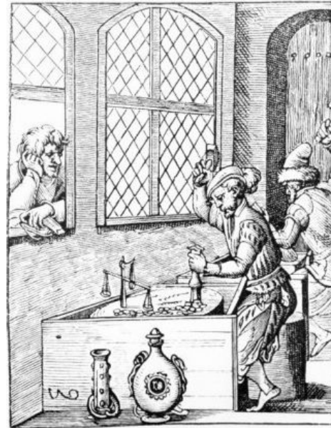
Figure 1: "Der Münzmeister", xylography by Jost Amman (1568), representing the hand-hammering work in an ancient mint.
