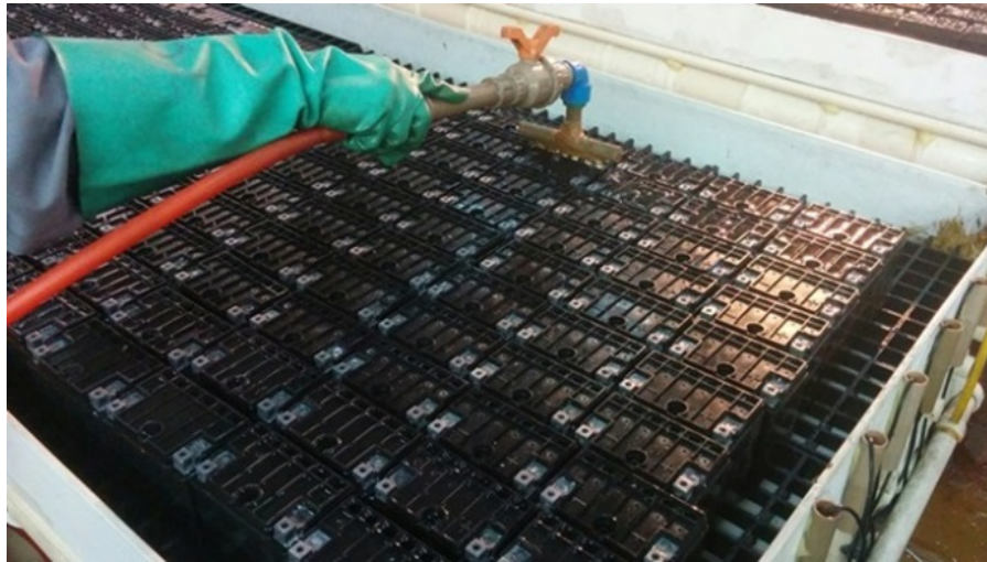
Figure 1: Initial step of the formation process: filling.
