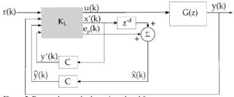
Figure 5. Proposed control scheme in a closed form. Source: The authors.
