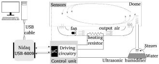
Figure 8. Schematic diagram of the incubator unit prototype. Source: The authors.
