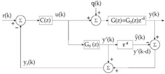
Figure 3. Discrete-time Smith predictor structure. Source: The authors.
