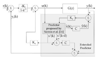
Figure 4. Proposed control scheme with modified dead-time compensation. Source: The authors.
