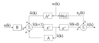
Figure 1. Explicit dead-time compensation structure (predictor). Source: Adapted from [16].
