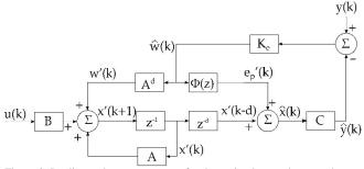
Figure 2. Predictor-observer structure for the optimal control approach. Source: The authors.
