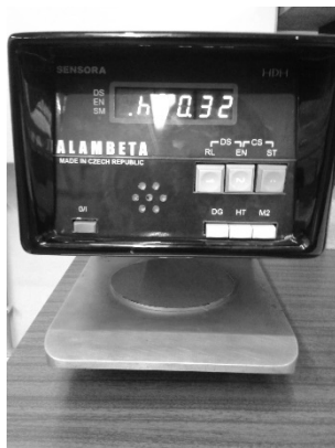
Figure 1 Alambeta equipment for thermal properties measurement Source: The authors
