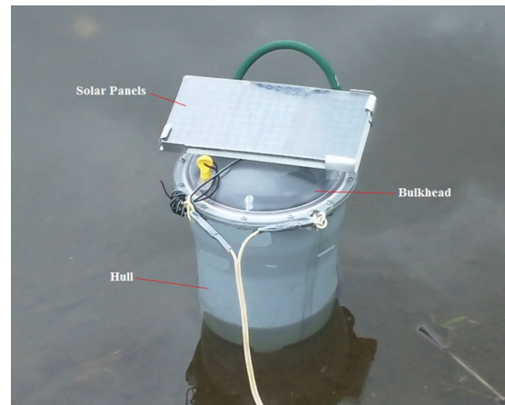
Figure 8. Buoy station prototype field test.
