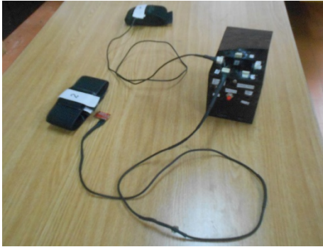
Figure 2. Final prototype. Top figure: Control unit that includes a 32-bit microcontroller, an XBee module, a LIPO battery, and connectors and LEDs indicators. Bottom figure: arm straps, IMUs and cables connected to control unit.
