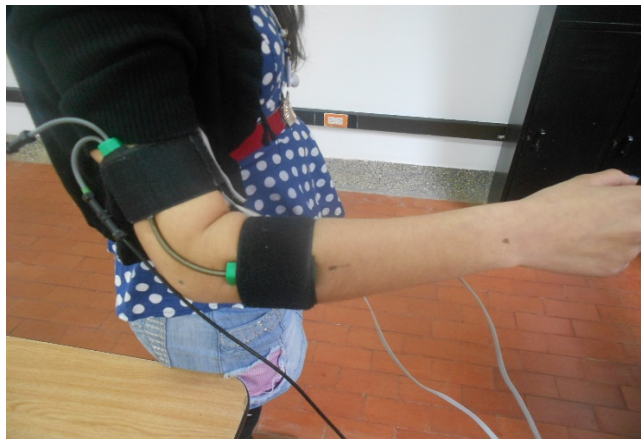
Figure 5. Inertial sensor-based electrogoniometer and SG110 commercial electrogoniometer was worn to measure flexion-extension angle. Source: The authors.
