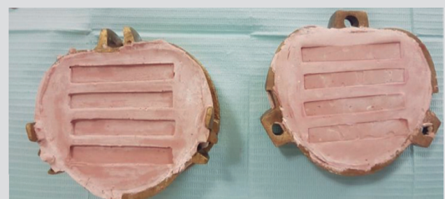
Figure 2. Patterns that leave the wax in the extruded gypsum using the lost wax technique.
