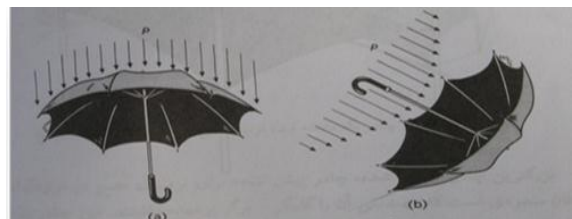
Figure 2. Pre-tensioned membrane, an umbrella (Mohammad Mujahidin,2015)
