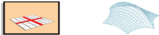
Figure 4. Saddle form an arch support across the membrane by structures placed in a stretched position (Mahmoud et al 2013)
