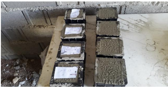
Figure 2 Control and nano sampling of fresh concrete
