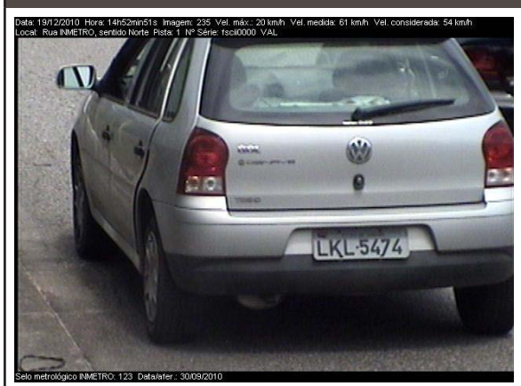
Figure 9. Photographic record generated by the instrument with the usual camera setup responsible for issuing registration.
