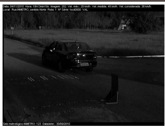
Figure 6. Photographic record generated by the instrument, configured with sensitivity level of 0.02%, for the test vehicle passing at 80 cm from the sensor.
