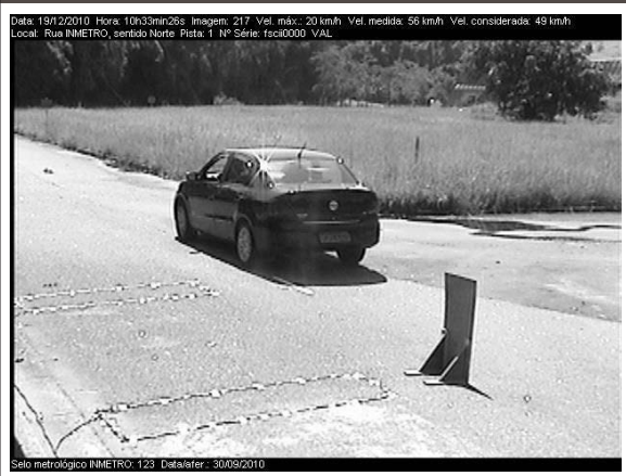
Figure 7. Photographic record generated by the instrument, configured with sensitivity level of 0.01%, for the test vehicle passing at 100 cm from the sensor.
