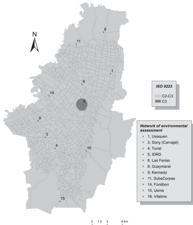
Figure 6. Map of atmospheric corrosion of carbon steel in Bogota, year 2011, according to ISO 9223 standard. Source: The authors
