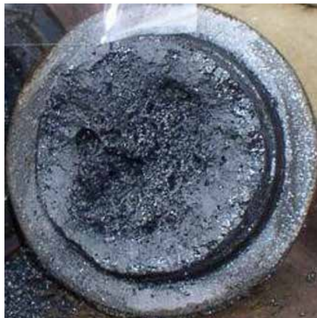
Figure 17. Coke sample extracted from a delayed coking pilot plant, Trigo (2005).
