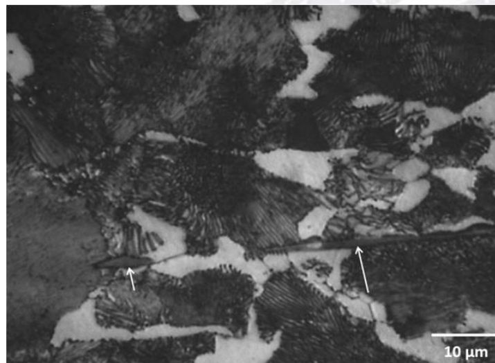
Fig. 11 SEM micrograph showing a MnS inclusion located along a grain boundary.
