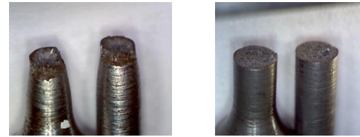
(a) Non-nitrided test specimen, ductile fracture (b) Nitrided test specimen, brittle fracture
