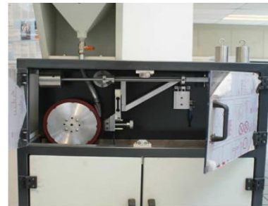
Figure 7 Abrasive wear machine.
