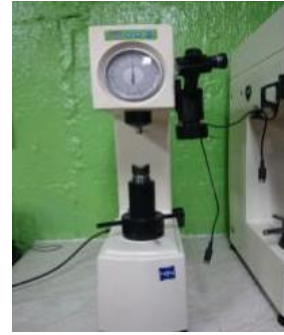
Figure 5 Hardness tester THBRV – 187_5D.
