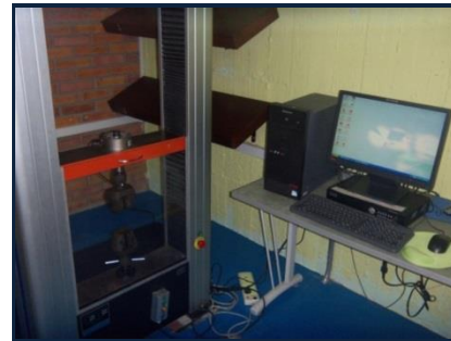
Figure 6 Universal testing machine. Microcomputer Controlled WDW-20E.
