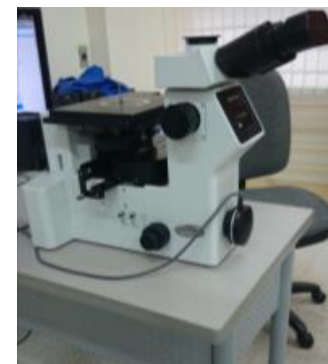
Figure 3 Olympus GX-71 metallographic microscope.
