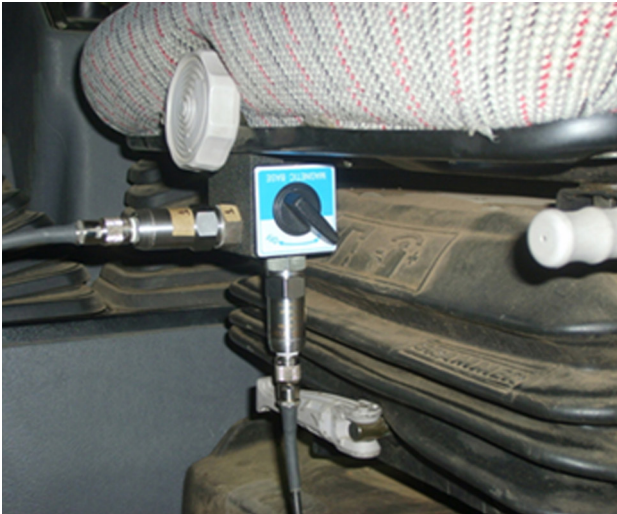
Figure 1. Setup for measuring vibration in the Zm and Xm axes.
