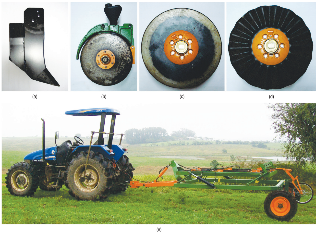
Figure 1. Furrow openers, coulters and motor-mechanic set: Hoe furrow opener (a), mismatched double-disc furrow opener (b), smooth coulters (c), offset fluted coulters (d) and set tractor and mobile tools holder (e).
