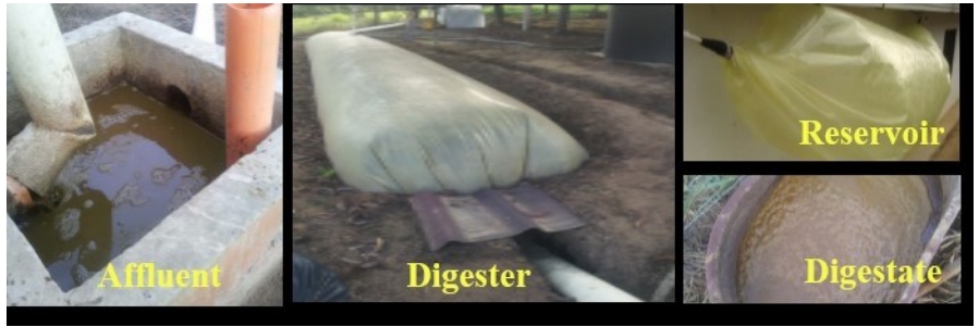
Figure 1. Tubular digester setup located on "Marcella" farm.
