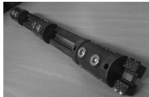
Figure 11. Carbon fiber rail assembled with commercial Lon Model clamps from Orthofix. Source: [7].
