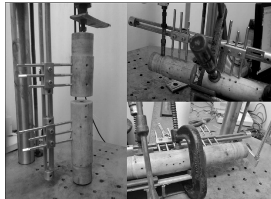
Figure 12. Custom made external fixation system used for comparing the stiffness. Source: The authors.
