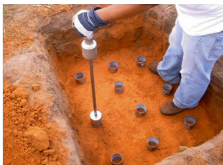
Figure 2. Soil removal carried out with the Umland sampler at different depths.
