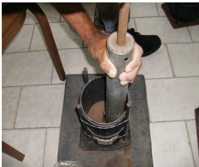
Figure 2. The employed experimental unit and the Proctor hammer in the infiltration analysis
