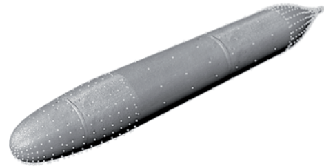
Fig. 4. Example of point cloud (white) obtained after digital image processing.
