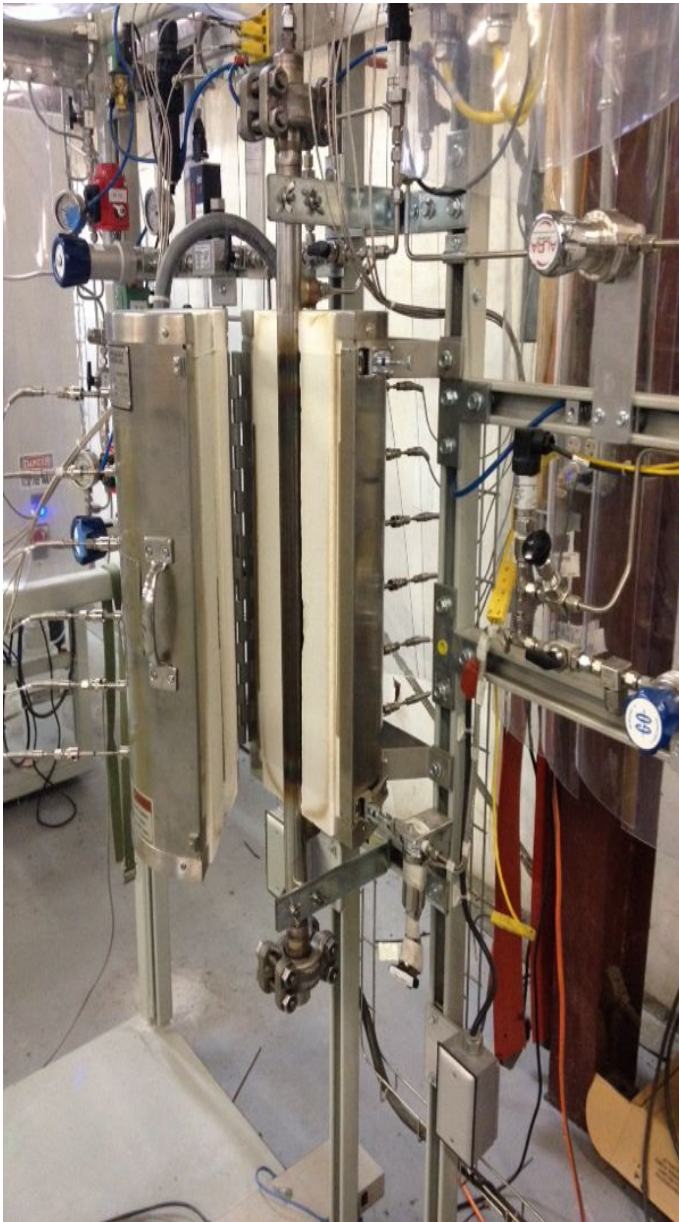
Figure 2. Oxidation Reactor with Temperature Ramp, ICP.
