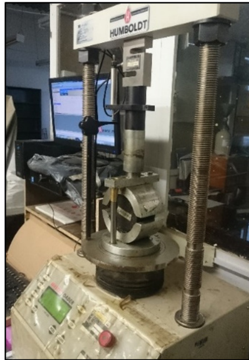
Figure 6. Equipment and test Stability and Marshall Flow
