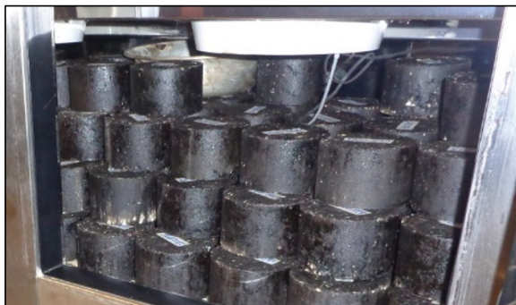
Figure 5. Experimental stage briquettes subjected to minimum freezer temperature
