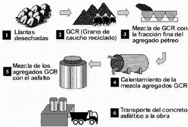
Figure 4. GCR Addition Process - Via Seca Fuente. Universidad de Los Andes (2002). Study of the mechanical improvements of asphalt mixtures with tire waste. Final report contract IDU-366-01. Alcaldía Mayor de Bogotá D.C.
