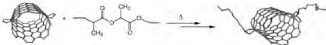
Figure 3. Reaction of a DCA functionalized CNT with PLA yielding the polymer functionalized CNT.
