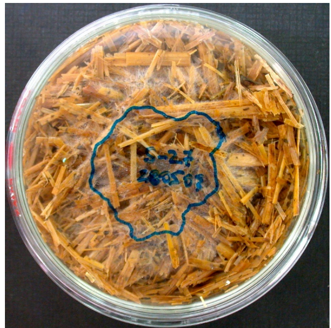
FIGURE 1. Drawing the mycelial area developed on the substrate, for its subsequent digitalization.
