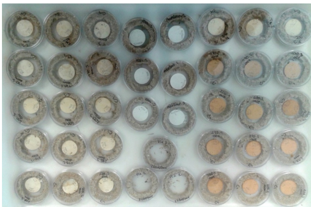
Figure 2: Termite screening test set-ups at the start of termite exposure.
