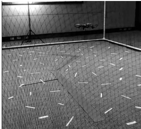
Figure 13. Photograph of the track and the Parrot minidrone following it.
