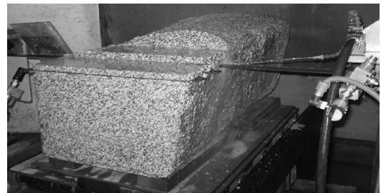
Figure 9. Brown granite cutting in progress
