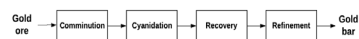
Figure 1. Generic process diagram for treating minerals that contain gold. Source: The Authors.
